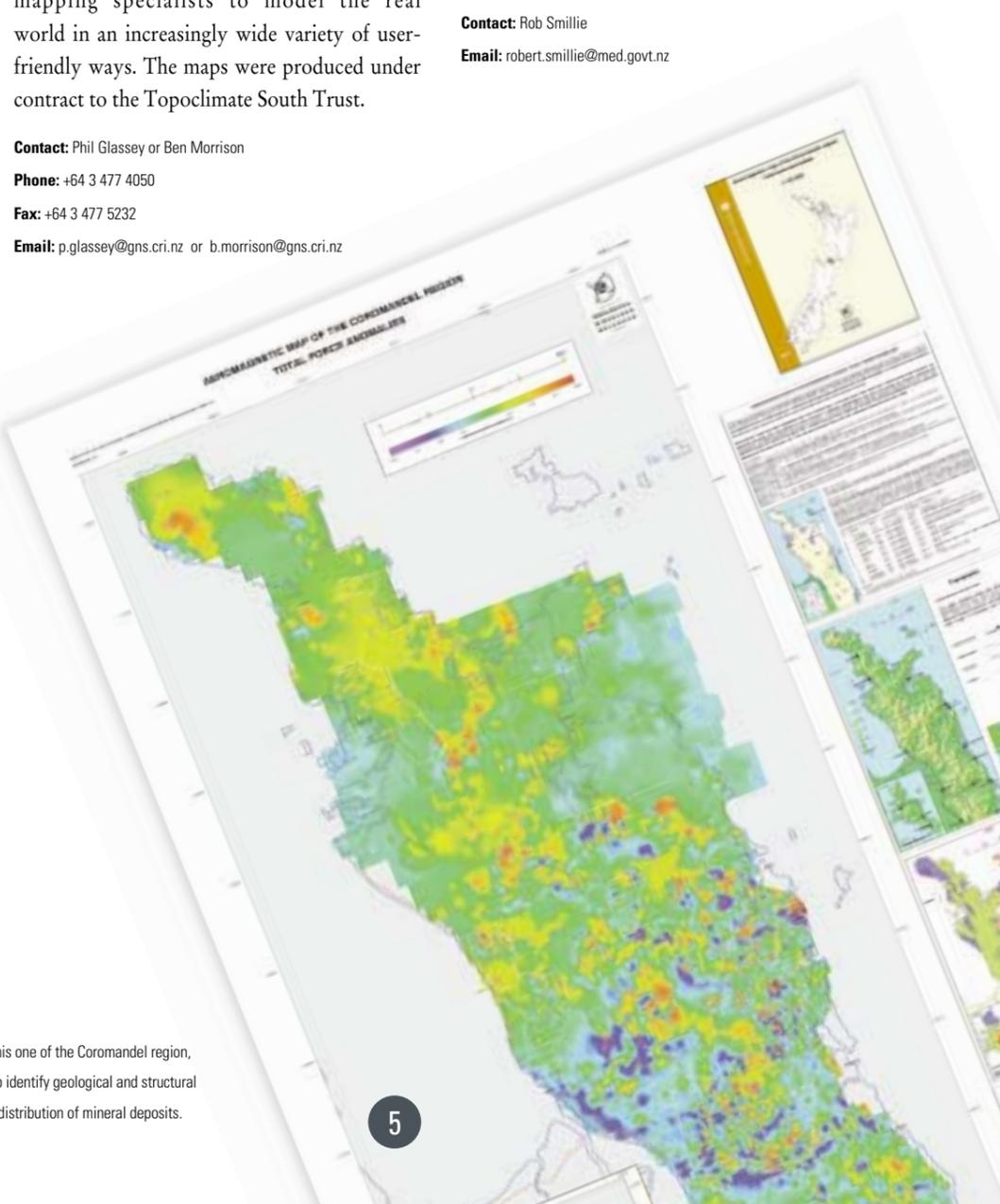
(Right) Aeromagnetic maps, such as this one of the Coromandel region, are used in mineral exploration to help identify geological and structural features that control the location and distribution of mineral deposits.
