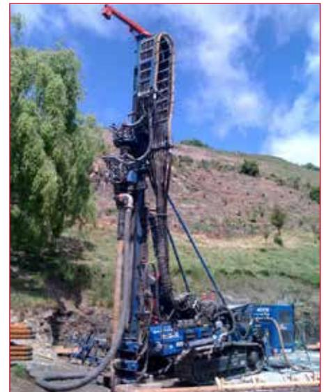
A drilling rig is needed on site to install a vertical ground source system.
