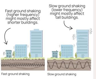
This is why we have seen some buildings affected more than others in previous earthquakes. Buildings move as a result of the unique combination of earthquake source, ground shaking, soil type, and building design.
