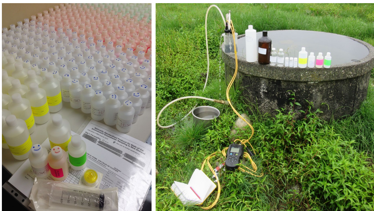
Figure 2.1 Photos of the NGMP sampling kit for chemistry prepared at NZGAL (left) and deployed in the field (right). The chemistry set consists of four Nalgene® sampling bottles: yellow label, green label, pink label and white label. Bottle caps for pre-acidified bottles are marked to prevent the swapping of bottle caps in the field. The additional seven bottles shown in the field (right) are collected for age-tracer analysis, undertaken at the GNS Science Water Dating Laboratory. The latter samples are not collected quarterly.
