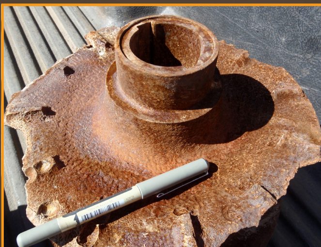
Ash-laden wastewater will cause accelerated damage to pump impellers (metal pitting and thinning).
