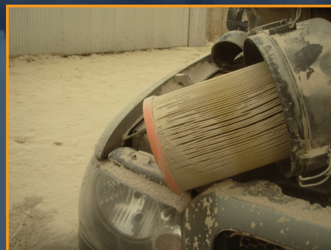
Heavy ash contamination of car air filter following 50 mm of ashfall from the 2011 eruption of Cordón Caulle volcano, Chile. (photo credit: Ailen Rodríguez, Jacobacci, Argentina)
