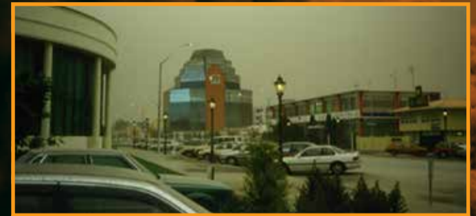
Rotorua CBD at 11:30 am on 17 June 1996, following an eruption of Ruapehu volcano earlier that morning. A layer of ash is visible on vehicles. Visibility is approximately 1 km (compared to clear air visibility of 70 km). Airborne ash concentrations were not measured but were likely in the range 0.1–0.5 mg/m 3 as PM 10 . In these conditions, high spec filters may need replacing every few hours to days, and low spec filters every few days to weeks. Photo: Rotorua District Council
