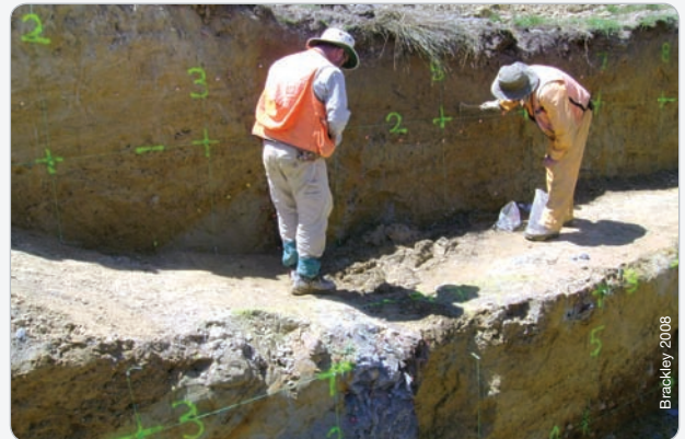
Trenching across faults reveals their earthquake histories.
