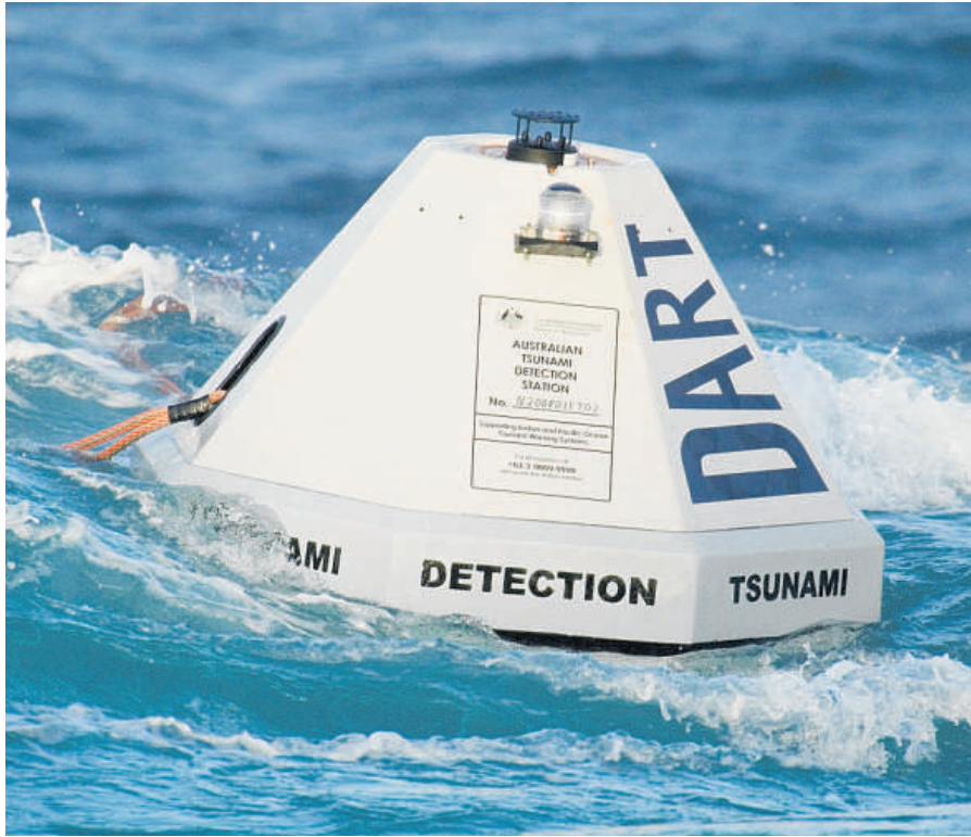
Dart buoys are positioned around the Pacific, providing real-time tsunami data (left). The tsunami buoy transmitting and receiving systems and sensors are tested and configured before deployment.
