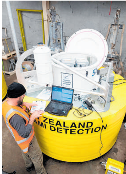
Dart buoys are positioned around the Pacific, providing real-time tsunami data (left). The tsunami buoy transmitting and receiving systems and sensors are tested and configured before deployment.
