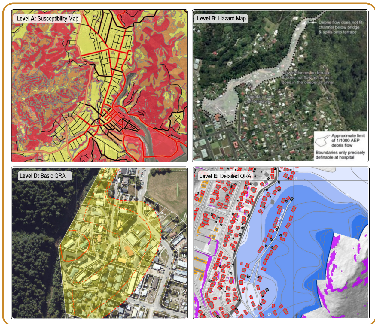
Figure 4.7: Example maps displaying the different levels of landslide susceptibility, hazard and risk analysis. Level A: Landslide susceptibility map of Whangārei District (Tonkin & Taylor 2022). Red, orange and yellow colours represent high, medium and low areas of landslide susceptibility. Runout has not been included in this map. Level B: Landslide hazard map showing the probability of a 1-in-1000-year AEP debris-flow event impacting the Thames Hospital (McSaveney and Beetham 2006). Level D: Basic quantitative risk assessment example, where debris-flow AIFR from three scenarios (small, moderate and large debris flows) was calculated for Gorge Road, Queenstown. 16 Level E: Detailed quantitative risk assessment example, where rockfall AIFR risk is calculated for the full range of earthquake and non-earthquake triggers that could occur in the Port Hills, Christchurch (Massey et al. 2012).
