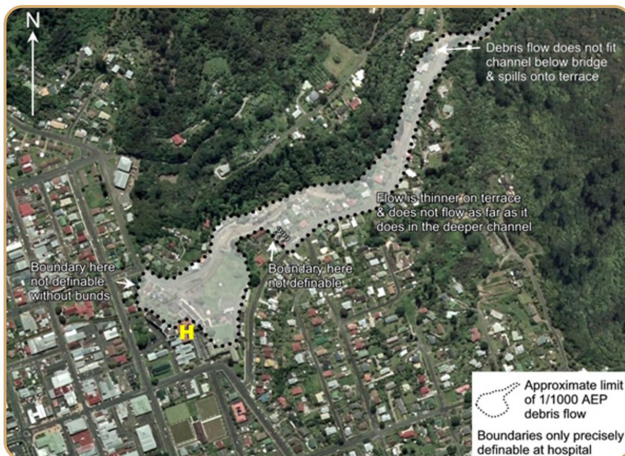
Figure 7.3: Example of a landslide hazard assessment that includes risk. The annotated aerial photograph depicts the 1-in-1000 AEP debris-flow hazard zone at Karaka Stream, Thames, Coromandel, in relation to existing Building Importance Level 3 buildings in the Thames Hospital complex (H).
