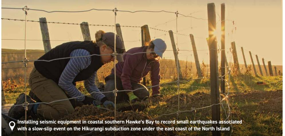
Installing seismic equipment in coastal southern Hawke's Bay to record small earthquakes associated with a slow-slip event on the Hikurangi subduction zone under the east coast of the North Island
