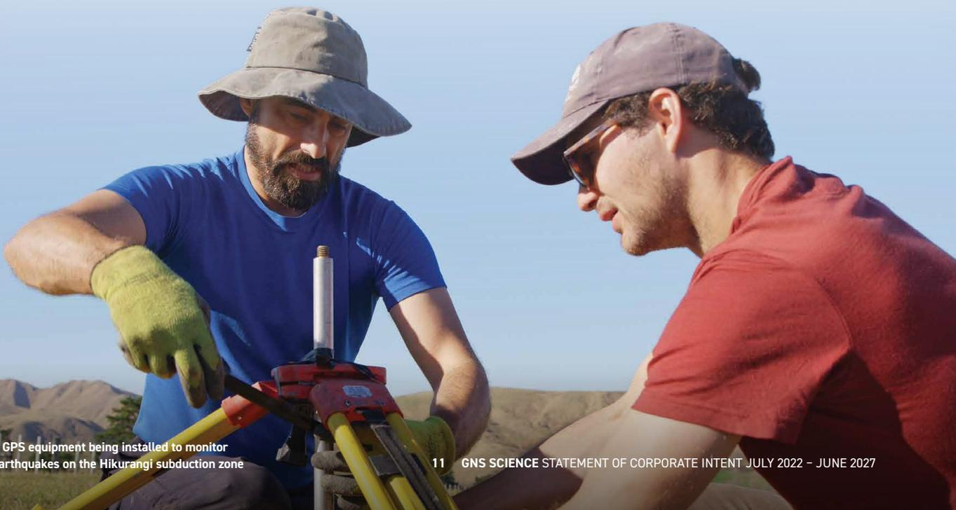
Temporary GPS equipment being installed to monitor slow-slip earthquakes on the Hikurangi subduction zone
