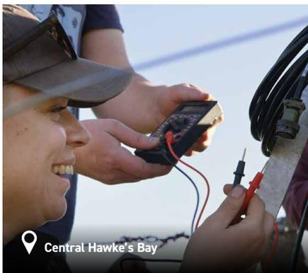
Checking the voltage of a solar panel being used to power a seismometer station
