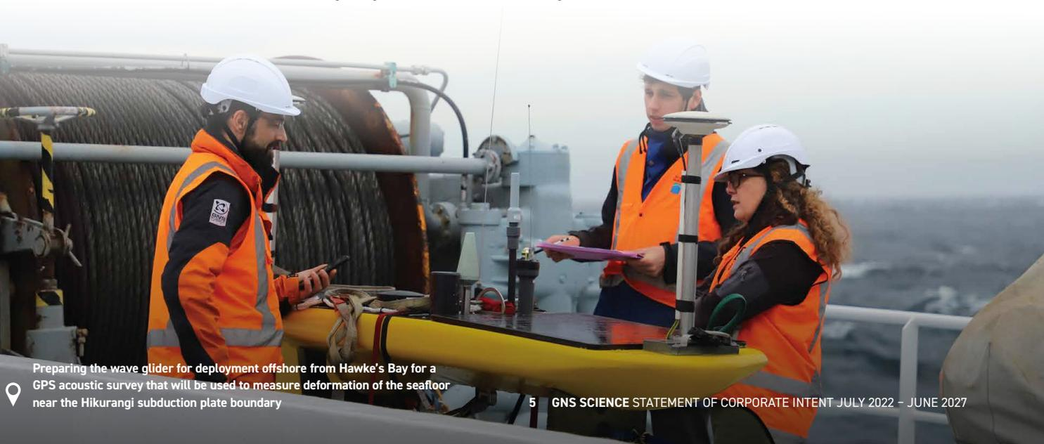
Preparing the wave glider for deployment offshore from Hawke's Bay for a GPS acoustic survey that will be used to measure deformation of the seafloor near the Hikurangi subduction plate boundary
