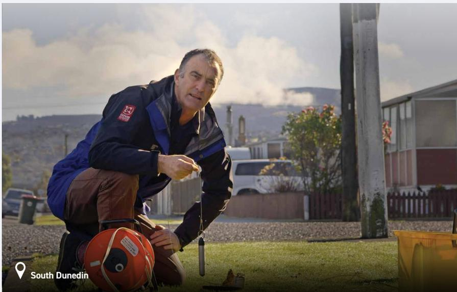
Using an electronic tape to measure the depth to groundwater at a monitoring borehole. Sitting just 50 cm below the surface, the water table's response to extreme weather events and sea level rise is of great concern to the community
