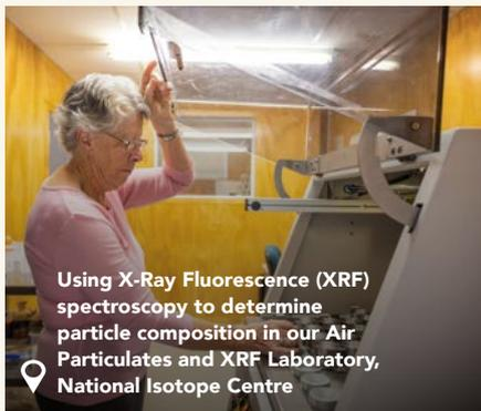
Using X-Ray Fluorescence (XRF) spectroscopy to determine particle composition in our Air Particulates and XRF Laboratory, National Isotope Centre
