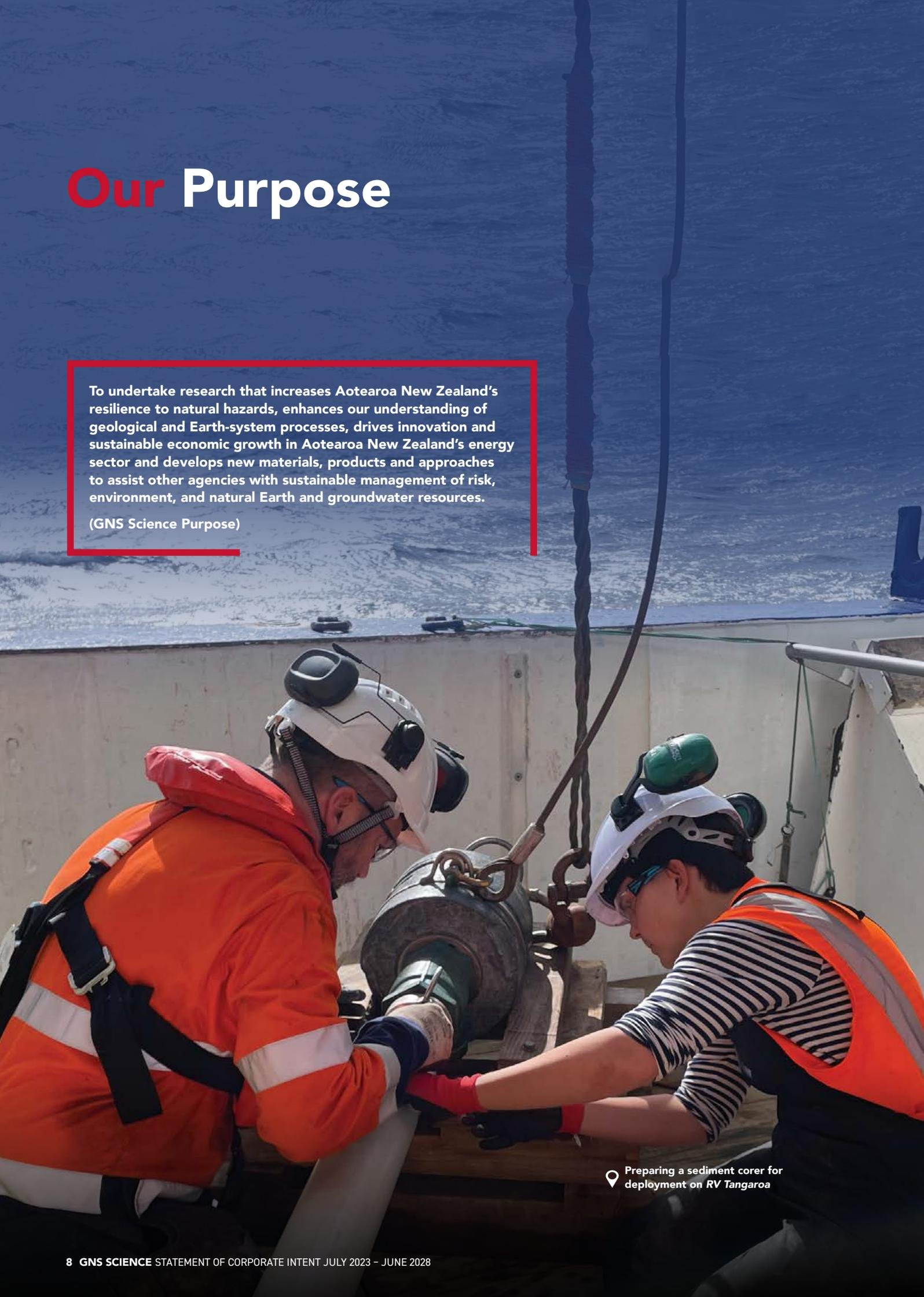
Preparing a sediment corer for deployment on RV Tangaroa
