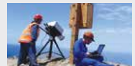
P26 Scientists use infra-red equipment to measure composition of gases being emitted from White Island crater – Karen Britten
