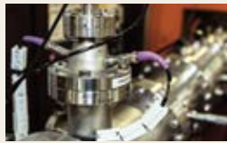
P53 Ion implanter beam line at the National Isotope Centre – Margaret Low, GNS Science
